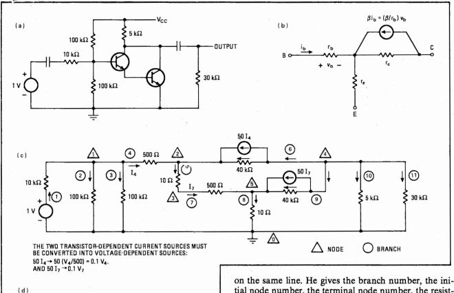
2. Program at work. The transistor amplifier in (a) is analyzed for dc conditions. The T-model equivalent circuit (b) can be used for the transistors, provided that all dependent current sources are converted into voltage-dependent sources. In the complete amplifier equivalent circuit (c), all nodes and branches are numbered consecutively. The program printout is shown in (d).
