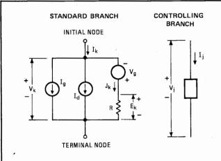
$$\begin{split} & v_k, \, v_j = \text{branch voltages} \\ & I_k, \, I_j = \text{branch currents} \\ & E_k = \text{element voltage} \\ & J_k = \text{element current} \\ & v_g, \, I_g = \text{independent sources} \\ & I_d = g_m \cdot v_i \, (\text{voltage-controlled current source)} \end{split}$$
